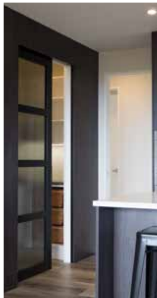
↑ 1 - CS NewYorker black powder coated 4-lite door with grey laminate glass.
