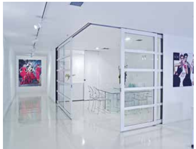
3 - White powder coated 5 horizontal lite CS NewYorkers with clear glass in corner meeting CS OvertakingDoors cavity sliders.
