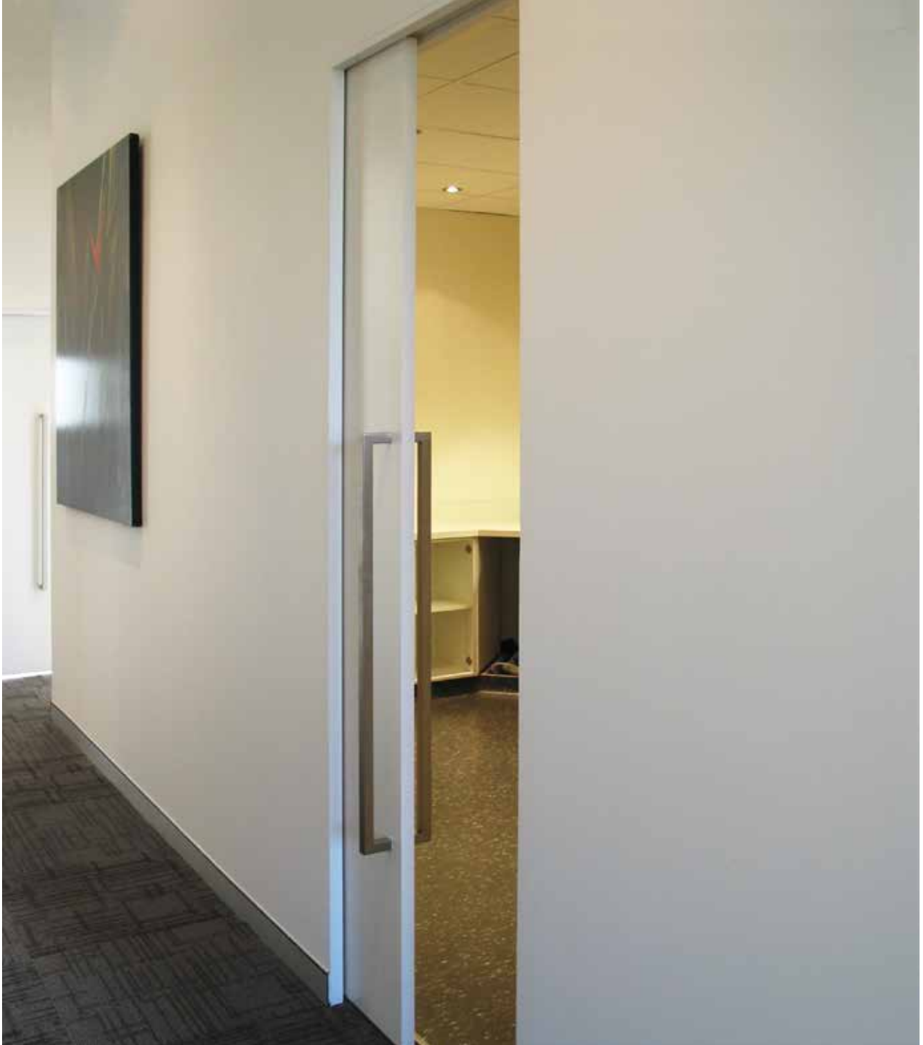
CS SoundStop Single unit with STC 42 / RW 42 dB door
