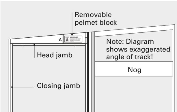
After installation but before lining, **clean the full length of the inside running surface of the track with a soft rag. TAPE UP THE TRACK to ensure no dust or debris enter the track or SofStop mechanism during building works.** Warranty does not cover damage arising from paint or debris in the track, wheels or mechanism.
